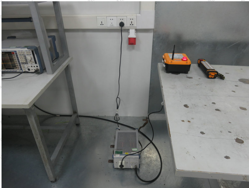
Photo of Conducted Emission Test
