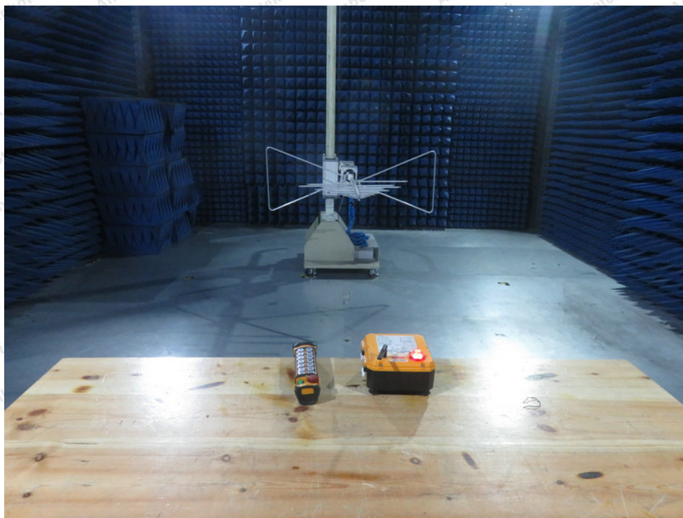
Photo of Radiation Emission Test
