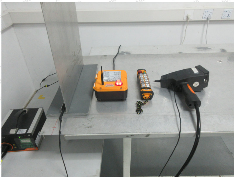
Photo of Electrostatic Discharge Test
